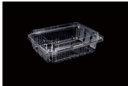
型号: JM-300B 装箱: 600个 材质: PET 尺寸: (外) 175mm*135mm*55mm (内) 160mm*118mm*53mm
